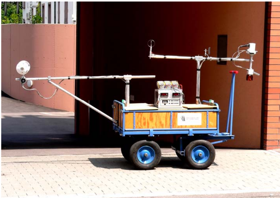
Fig. 4: Mobile human-biometeorological measuring system used in Freiburg
