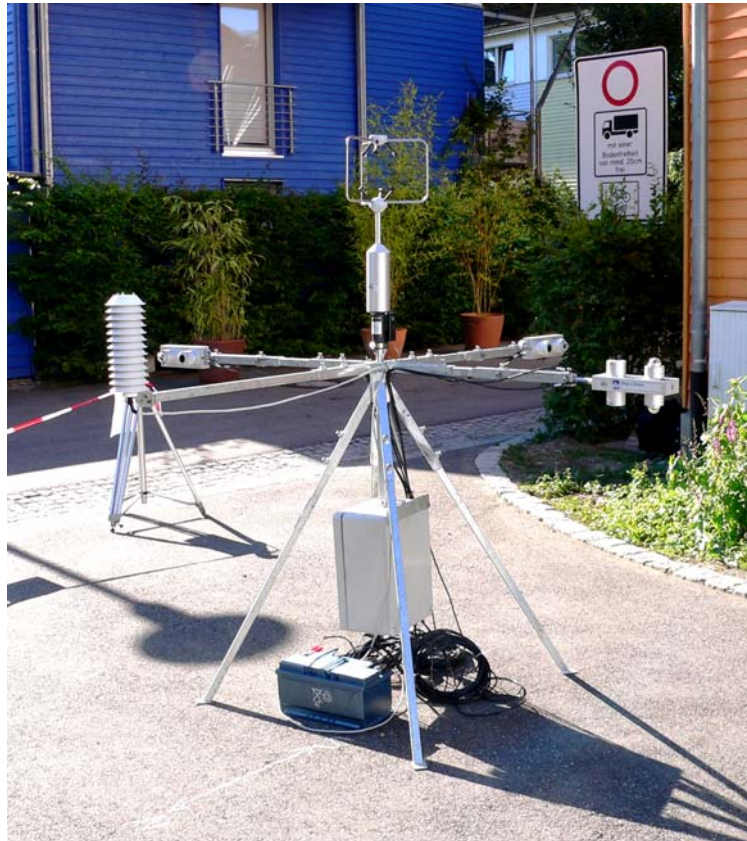
Fig. 3: Stationary human-biometeorological measuring system used in Freiburg
